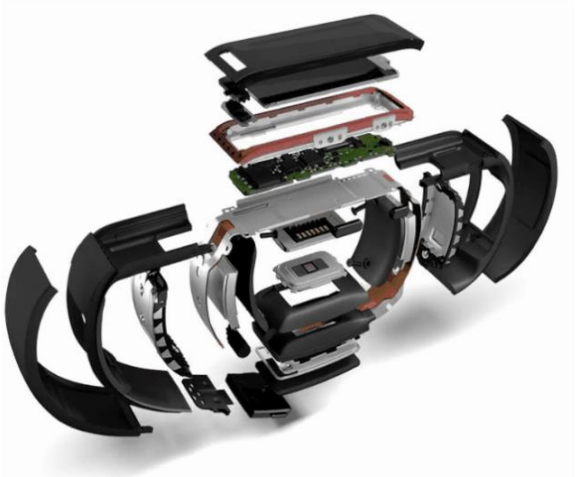
An exploded view of the Microsoft Band, a product similar to the oneBand Health Band.
